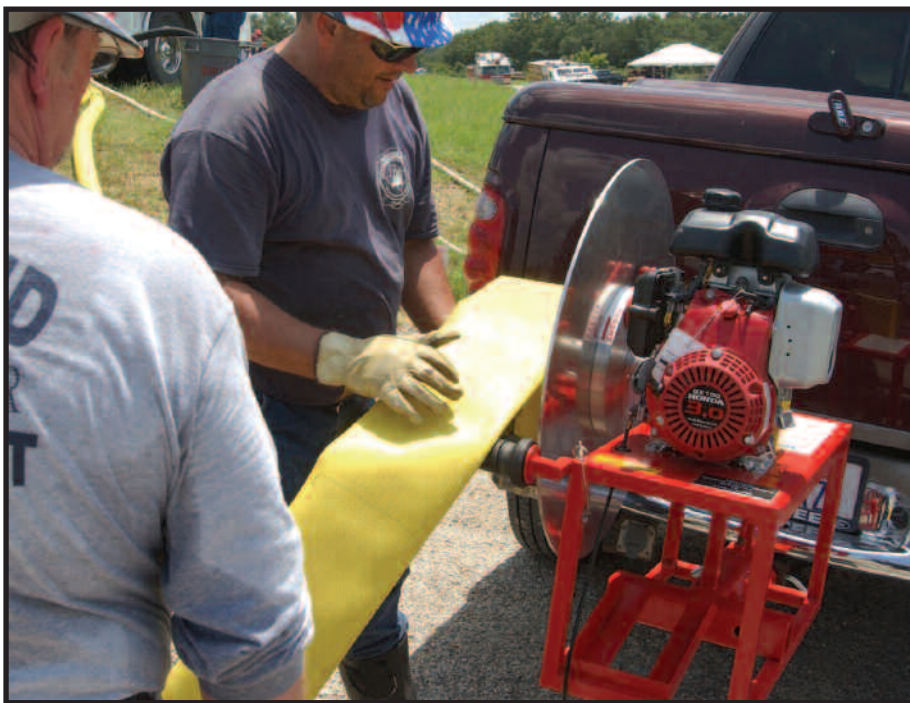
Instructors at Brayton Fire Training Field in College Station, Texas, put the Rookie Sidekick gasoline-engine driven hose winder to the test.
